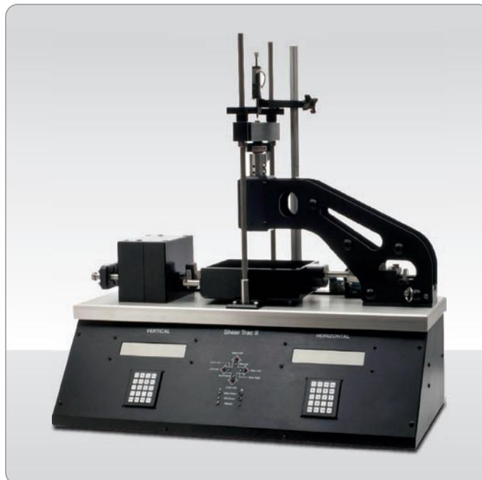
Standard Fully-Automated Rock Shear System
