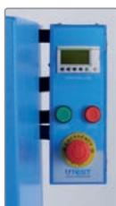
Start, stop, emergency stop buttons and digital counter are on control panel which is connected to the main body by anti-vibrating connections
