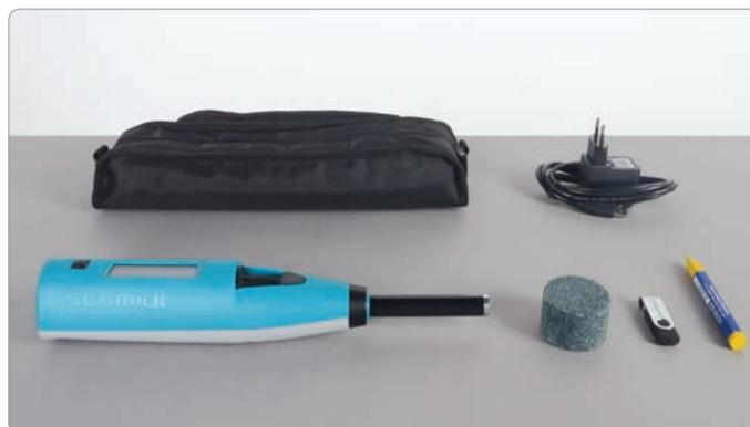
The Silver Schmidt Concrete Test Hammer is supplied complete with
